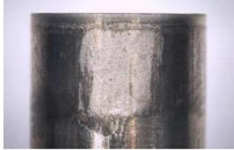
Figure 7. Stamping punch suffered severe galling
