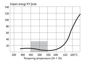
Tempering in the temperature range 450–550°C for the intended final hardness will result in a lower toughness.
