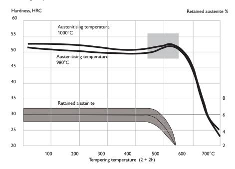
Above tempering curves are obtained after heat treatment of samples with a size of  $15 \times 15 \times 40$  mm, cooling in forced air. Lower hardness can be expected after heat treatment of tools and dies due to factors like actual tool size and heat treatment parameters.
